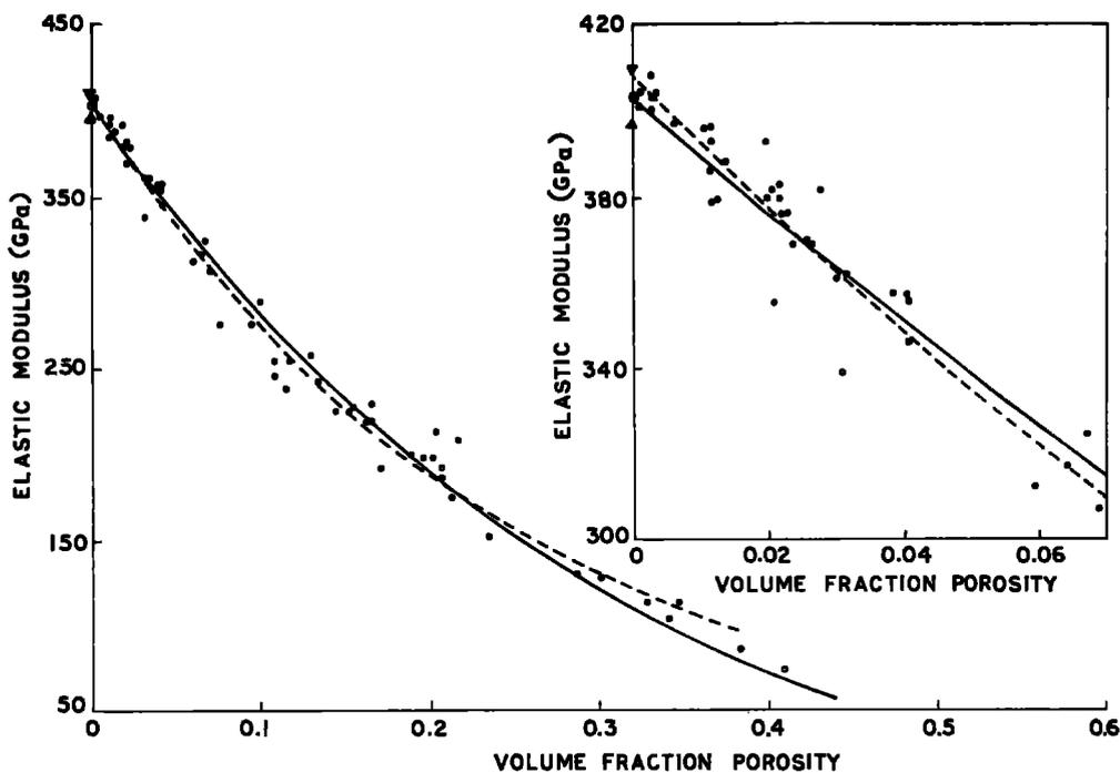
Figure 4 Young's modulus plotted against porosity of  $\alpha$ -alumina. A total of 71 data points as compiled by Knudsen [2] is shown in the plot. ( $\nabla$ ) Voigt bound, ( $\blacktriangle$ ) Reuss bound, ( $\circ$ ) Hill average. (---) Wang's equation, (—) proposed equation.
