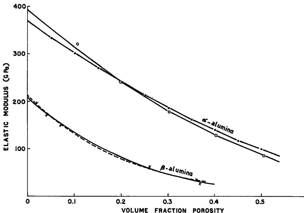
Figure 5 Young's modulus plotted against porosity of  $\alpha$ - and  $\beta$ -alumina. A total of 5 data points of  $\alpha$ -alumina as reported by Coble and Kingery (O) [8] and that of 6 data points of  $\beta$ -alumina as reported by Evans *et al.* (x) [9] are shown in the plot. (---) Wang's equation, (—) proposed equation, (— · —) Mackenzie's equation.
