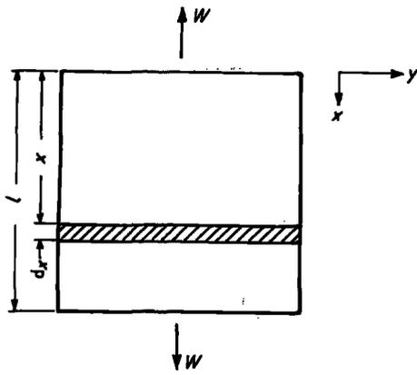
Figure 1 Porous body in tension: a schematic view.
