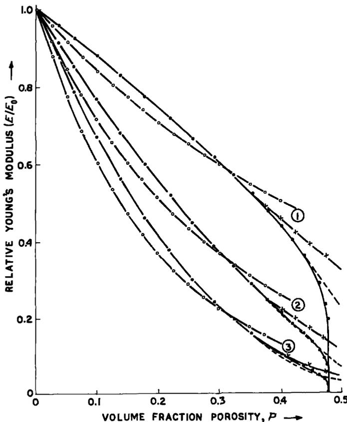
Figure 2 Young's modulus as a function of porosity. The exact solution ( $\bullet$ ), Spriggs' correlation ( $\circ$ ), Wang's correlation ( $\times$ ) and the proposed equation (---) are shown in the plot. (1) Ideal case, (2) non-ideal case (shear effect), (3) non-ideal case (combined shear and hinge effect).
