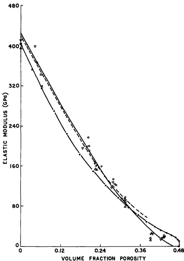
Figure 3 Young's modulus plotted against porosity of  $\alpha$ -alumina. A total of 37 data points as reported by Wang [7] is shown in the plot. ( $\nabla$ ) Voigt bound, ( $\Delta$ ) Reuss bound, ( $\circ$ ) Hill average. (---) Theoretical equation, (- -) Wang's equation, (—) proposed equation.
